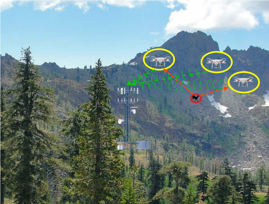
Figure 8-1 Habitat monitoring: a set of autonomous UAVs monitor the object of interest in an inaccessible area and collectively report their observations to a central ground station for further processing.
